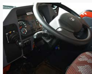
Tilt and telescopic Power Steering - Adjustable to any driver with respect to his height
