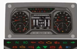
New Multifunction Instrument Cluster Features: Average Fuel Economy, Digital DEF indicator Gear Shift Advisor, Regeneration Indicator Tell Tale Symbols
